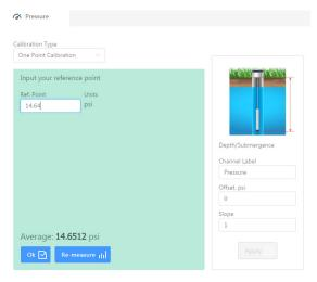
Click Ok to accept the reading and Aqua4Plus 2.0 will calculate a new pressure offset. Click Apply to confirm the new offset value and Aqua4Plus 2.0 will provide a real time reading to verify calibration was successful:
